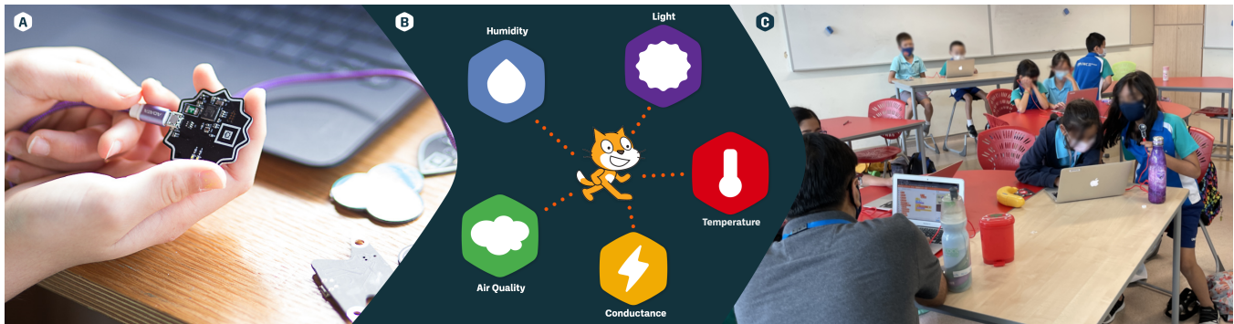
Figure 1: A) Our plug-and-play sensor toolkit tailored for use by young children; B) Seamless access to exploring physical phenomena and integrating real-time data with Scratch; C) Students engaging in free exploration with the toolkit.
