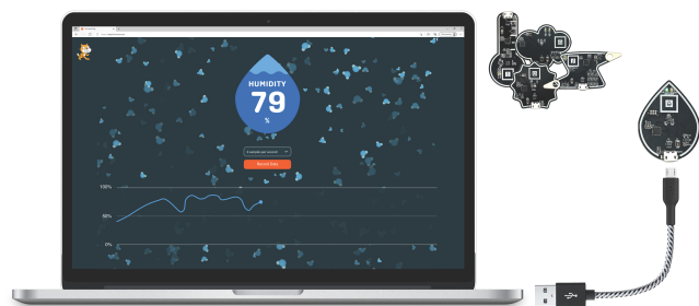
Figure 3: A standard Micro-USB cable makes for a simple connection between sensor and host device. Upon connection, the sensor type is automatically detected and data readings become available in the web browser.
