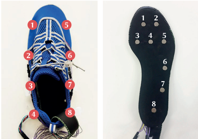
Figure 3: Left: Shoe prototype (UK size: 10-11). The sensing.tex FSR-based plantar pressure insole is inserted and 8 vibration motors (ROB-08449) are attached at the inside of the shoe's wall. Right: 3D-printed insole Prototype (UK size: 10-11). The sensing.tex pressure insole is covered by a 6mm thick rubber layer (ninjaflex 85A filament) that incorporates 8 vibration motors.
