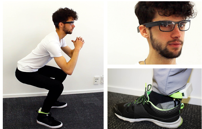
Figure 1: User performing squats with the GymSoles++ prototype. The pressure sensitive insole calculates the body's Center of Pressure (CoP). The insole also incorporates 8 vibration motors that map the CoP to vibrotactile feedback. The CoP is also visually displayed on a Google Glass.
