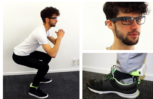
Figure 1: User performing squats with the GymSoles++ prototype. The pressure sensitive insole calculates the body's Center of Pressure (CoP). A rubber layer on top of the insole incorporates 8 vibration motors that map the CoP to vibrotactile feedback. The CoP is also visually displayed on a Google Glass.
