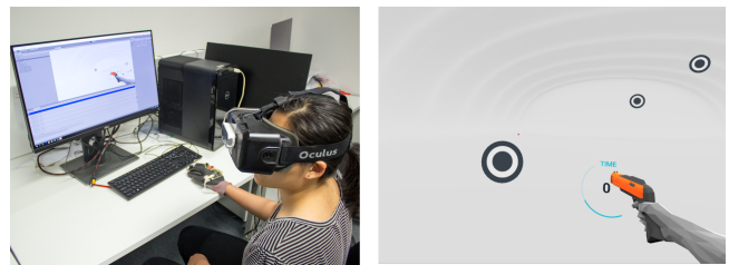
Figure 6: VR shooting game: the status of the ammunition and the recoil was provided via tactons.
