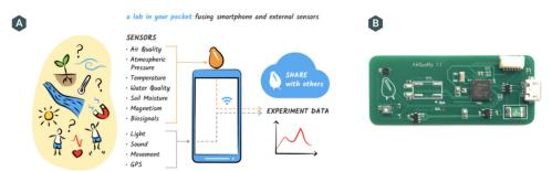
Figure 1. (A) The first concept of the mobile learning platform. (B) The first prototype of the pluq-and-play sensor used in Phase 1.
